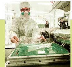
Example of the Gravure printing tool offering an efficient utilization of materials (additive manufacturing)
